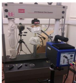
Figure 1: Experimental setup including hydraulic testing machine, infrared camera and visible camera.
