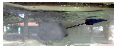
Figure 4. Developed cavitation in naval propeller
