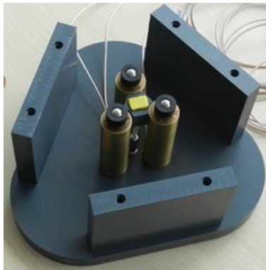
Prototype of a piezoelectric vibration assisted forging tool, with its nonlinear displacement versus voltage
