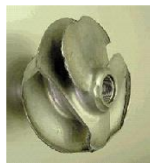
Figure 2. Hydrogen inducer of Japanese launcher H-II (after the flight failure)
