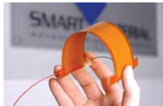
Figure 2: Macro-Fiber Composite piezoelectric device for vibration control ( https://spinoff.nasa.gov/ )
