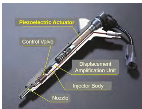
Figure 1: Common rail type diesel injection valve with a piezoelectric multilayer actuator (Denso Corporation, Uchino 2015)
